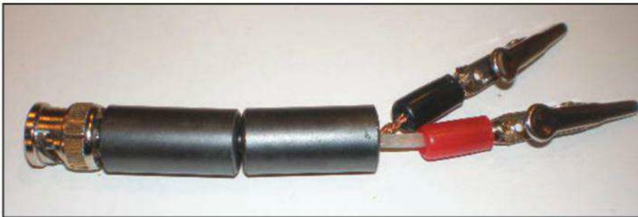
Photo B— An HF choke balun is essential for this type of antenna.
