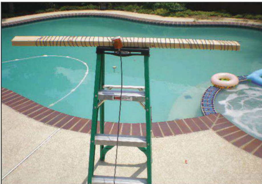
Photo A—Spiral antenna atop fiberglass ladder.
